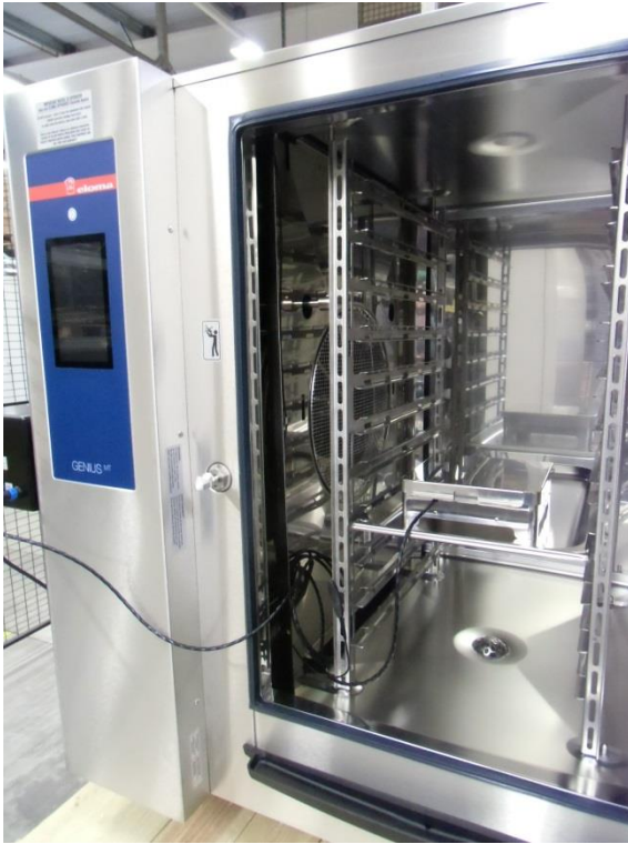
Fig. 2: Position of SmokeFit in the combi-steamer
